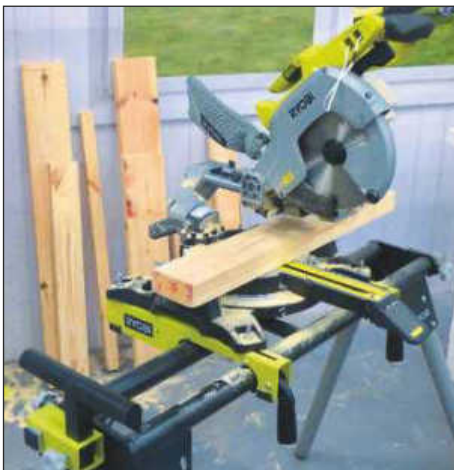
Although a prototype, this sliding mitre saw will run on two 18A batteries
